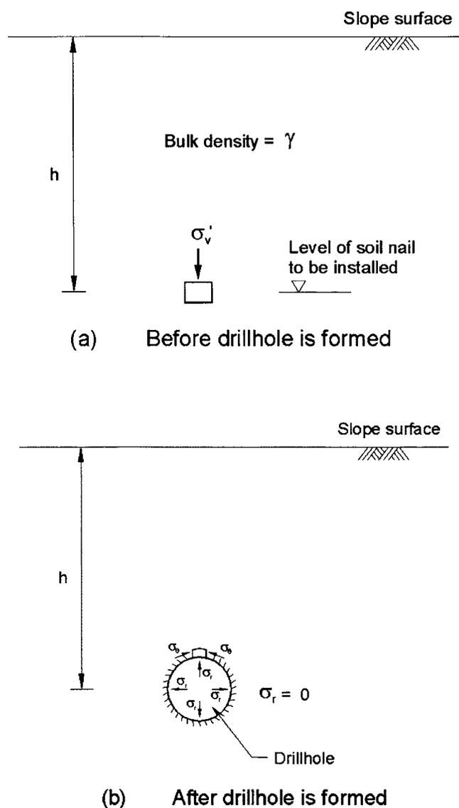
Fig. 1. Stress state around drillhole
