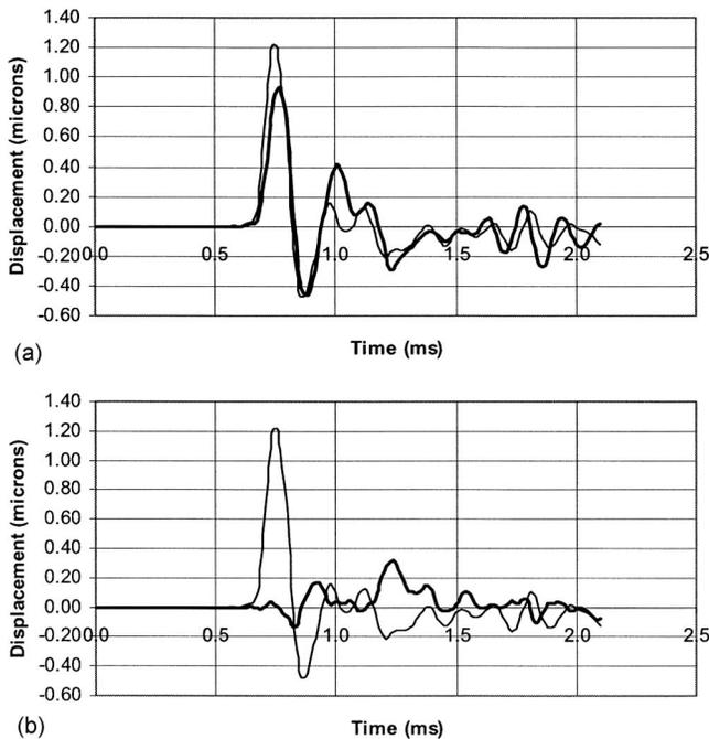
**Fig. 2.** Pile with no defect (thin line), with defect halfway between tubes (a), and with defect close to transmitter (b)
