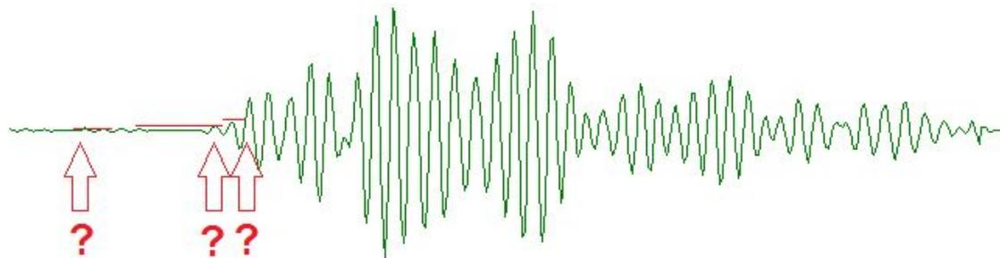
Fig. 5 - A typical ultrasonic wave with a gradually increasing amplitude
