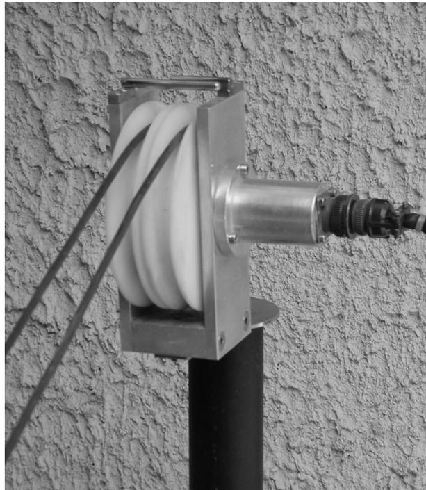
Figure 12: A double-wheel depth meter
