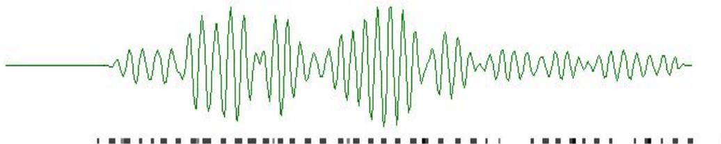
Figure 2 - Raw signal captured by a modern A/D (Analog to Digital code converter) and the corresponding waterfall pixel representation of the digital code
