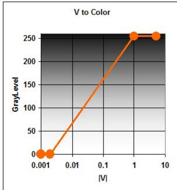
Figure 3 - Typical Voltage-to-Color mapping
